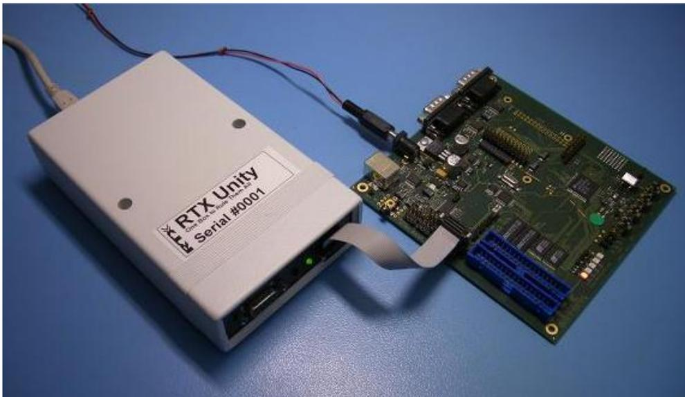
Figure 4. RTX Unity connected to CP3BT10 target.
