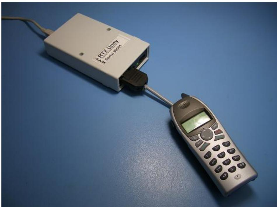
**Figure 3. RTX Unity connected to SC14428 target.**
