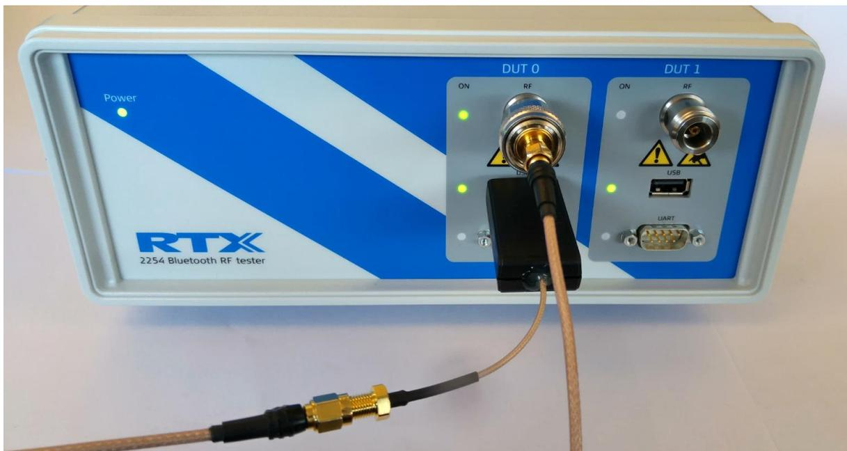
RTX2254 with "Test DUT" on USB
