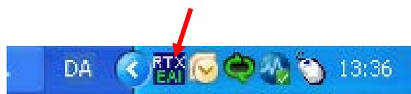
The Setup window can be opened by selecting **Setup** in the context menu. To open the context menu move the cursor to the REPS icon and click on the right mouse button (see below).
