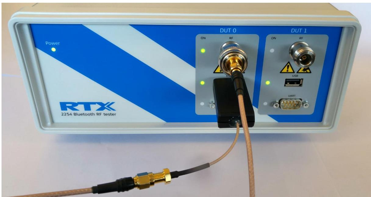
**"Test DUT"** is connected to DUT0 RF and USB
