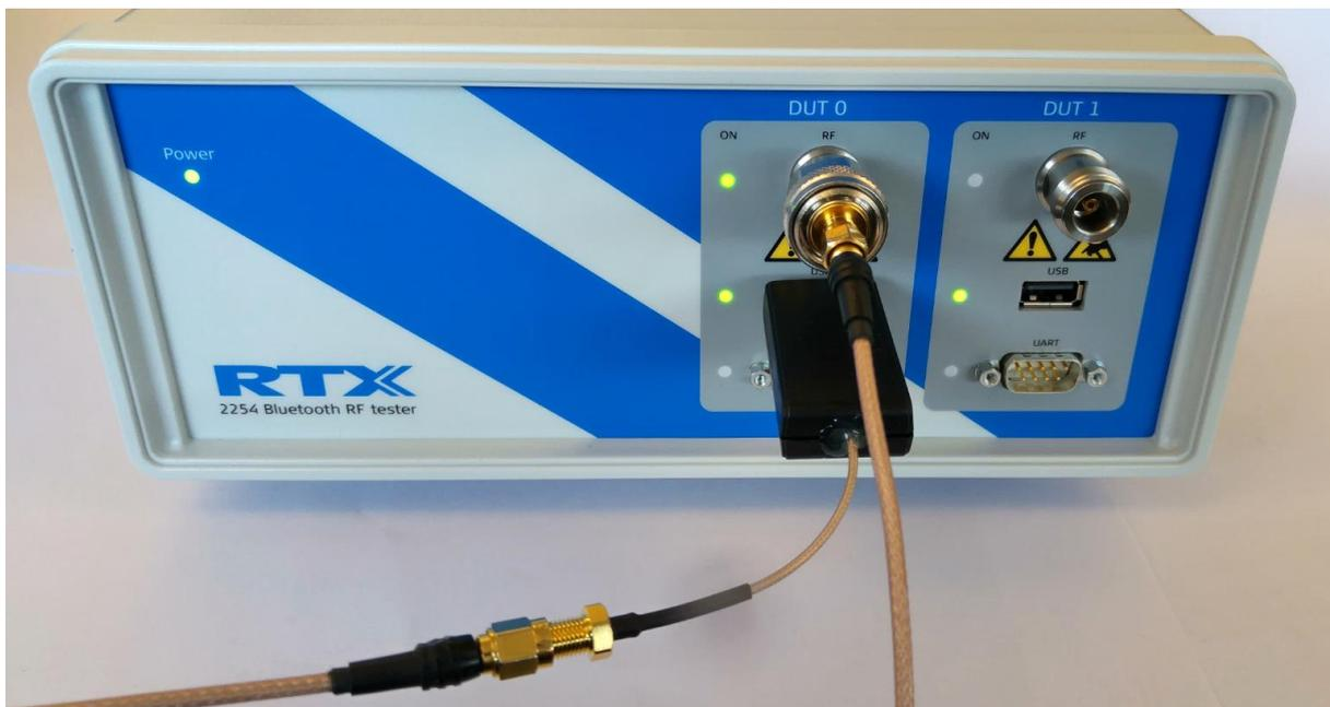
RTX2254 with "Test DUT" on USB
