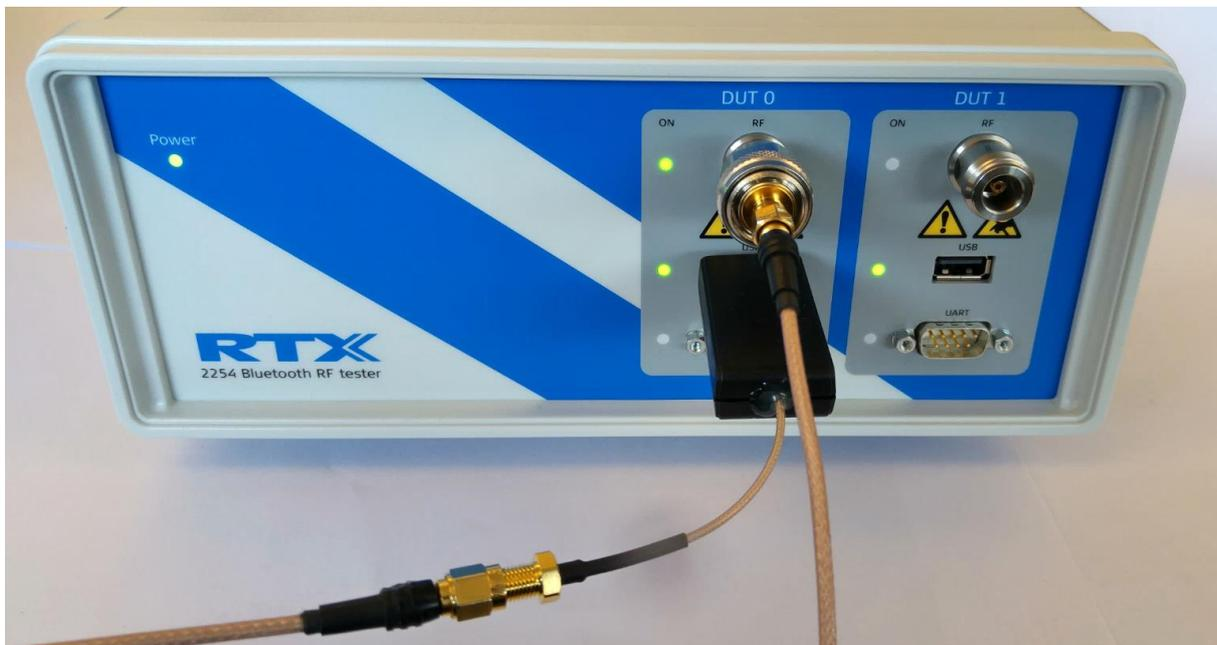
RTX2254 with "Test DUT" on USB
