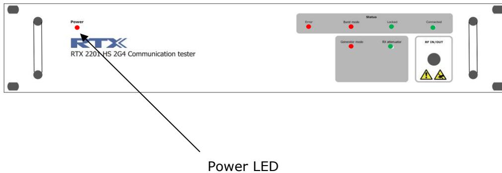
The Power On sequence indicates a functional running firmware.
