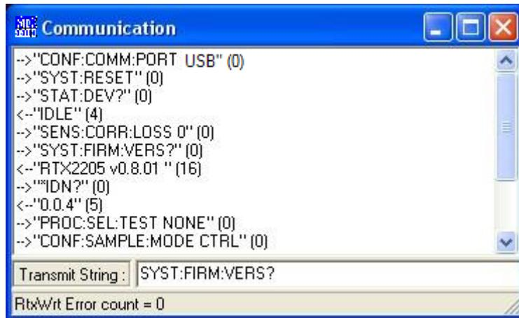
You can use this window to view and record the communication between your PC and test set, and send one command at a time in the **Transmit String** line. For more information about this feature refer to "Detailed Command Descriptions".
