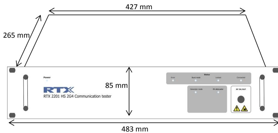
Place the Tester in the rack and secure it to the frame using four screws as shown below.
