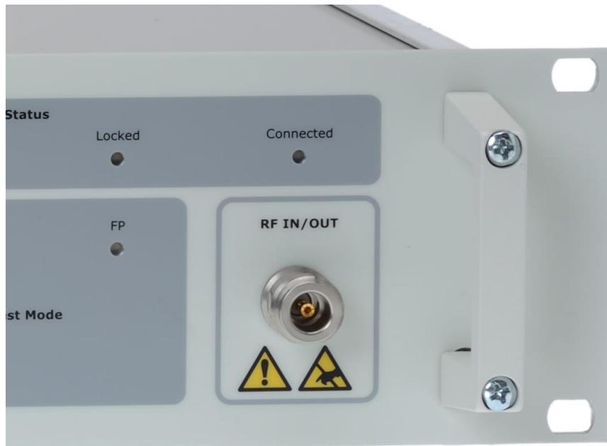
Make an RF cable connection between DUT and the RF IN/RF OUT connector.
