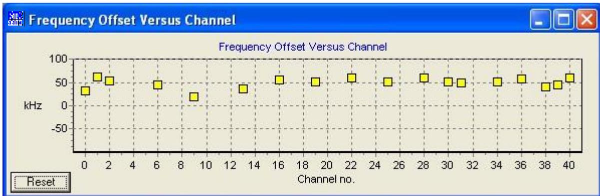
Like vice NTP measurements, Frequency Offset is measured and depicted for every channel measured.
