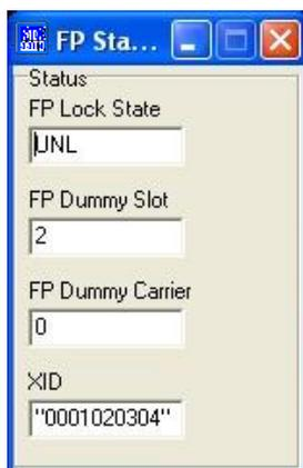
When the Tester is locked onto the DUT, the Status changes from UNL to LOCK.
