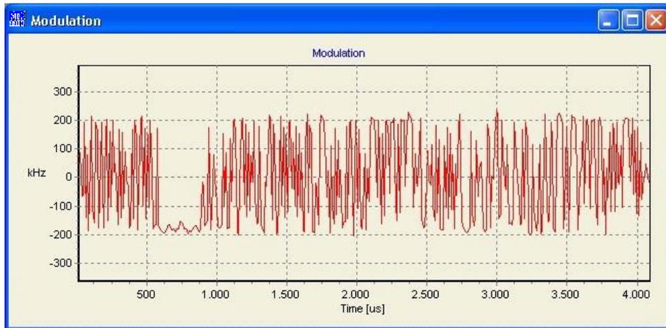
This modulation pattern is recommendable in sensitivity measurements.
