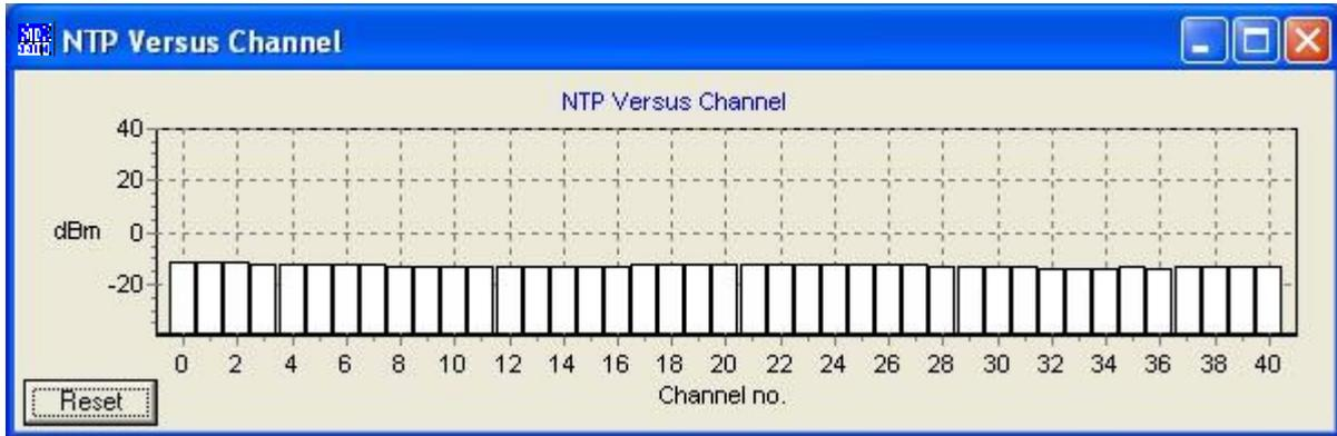
NTP is measured for each channel. The NTP vs. Channel display can be captured even when the DUT is changing frequency. Simply chose another channel to be visited. The Reset button erases the current measurements, and starts a new continuously data sampling.
