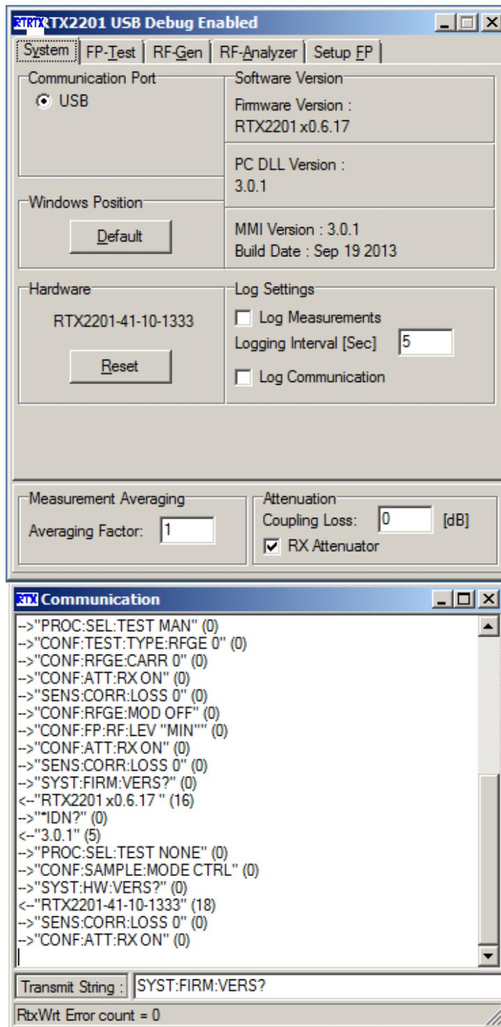
At the start of the commands showed in the communication area is an arrow showing the direction of the command e.g. an arrow pointing to the right --> is communication from the PC and an arrow pointing to the left <-- is reply from the test set. Returning a (0) means no errors, and (1) indicates a setting or communication error.
