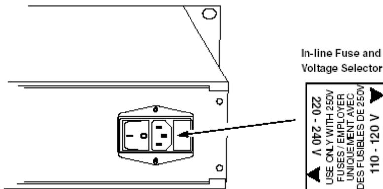
Select the required operating voltage by removing and replacing the fuse holder as shown below. Ensure the correct fuse is fitted.
