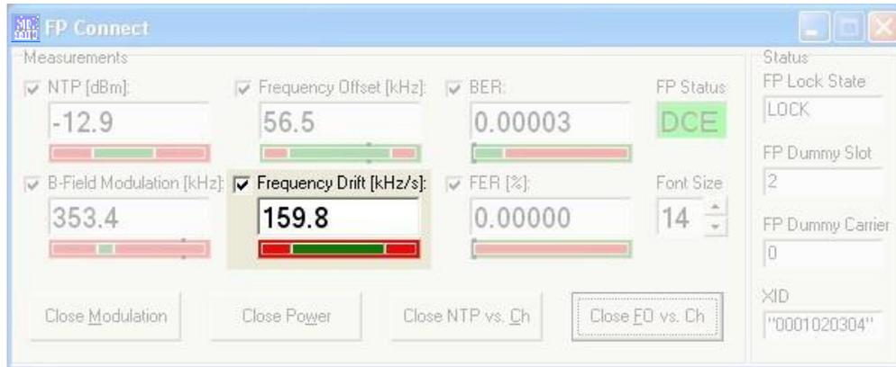
The Frequency Drift measurement can be read out by sending the remote SCPI command: **READ:FREQ:DRIF?**
