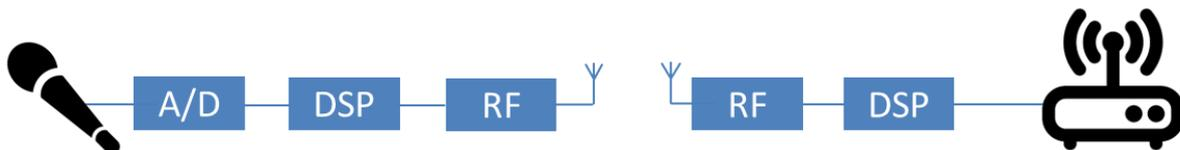
**Figure 1. A simplified architecture for a typical digital wireless microphone transmitter and receiver**
