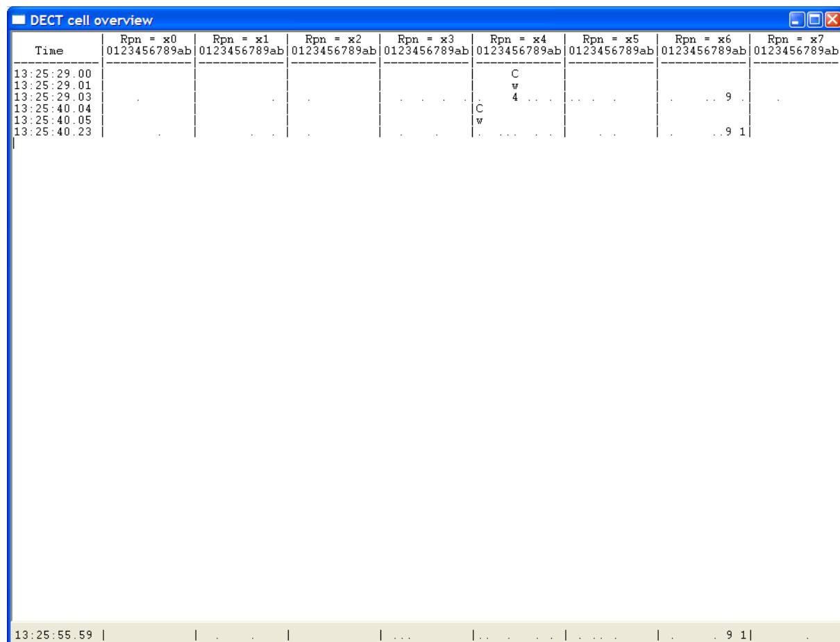
Show bearer activity in different cells (RPN mod 8). The activity in the individual slots are shown in separate columns (12 columns per RPN)
